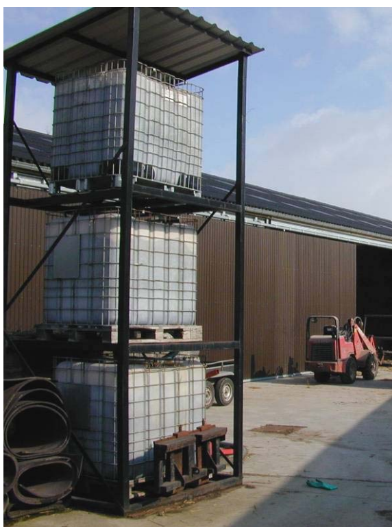
Fig.4: Biofilter (Bron: CRAw)
